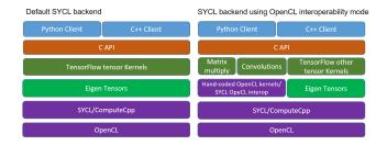
Figure 1: TensorFlow architecture for SYCL back-end
